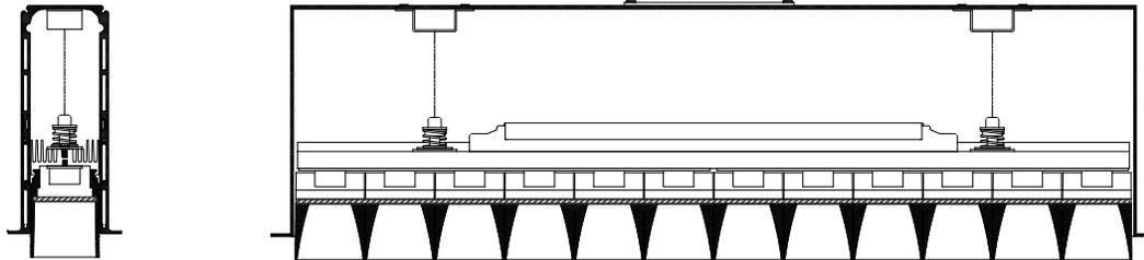
2. With LED assembly removed install housing as shown with screws through housing into blocking installed above. Pull power and dimming leads through wiring access plate with approved conduit connector. (FIG B)
