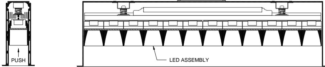
1. Remove lamp assembly from housing by pushing lamp assembly into housing releasing assembly from latch. (FIG A)
